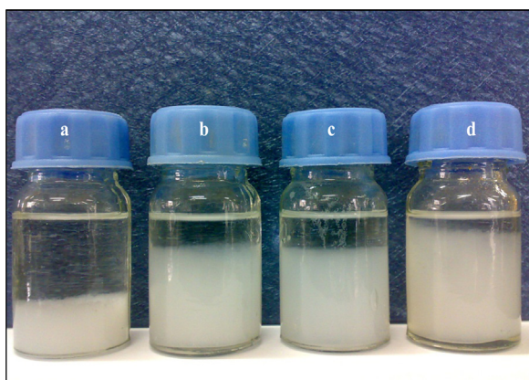
Fig. 2. Dispersion stability of the (a) native CNFs in acetone, (b) acetylated CNFs in acetone, (c) native CNFs in ethanol, and (d) acetylated CNFs in ethanol.
